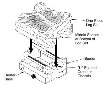
Figure 14 - Installing One-Piece Stove Log Set
